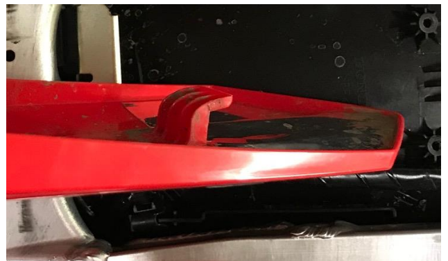
hooked tab that locks the underside of the outer fender into the rear fender
